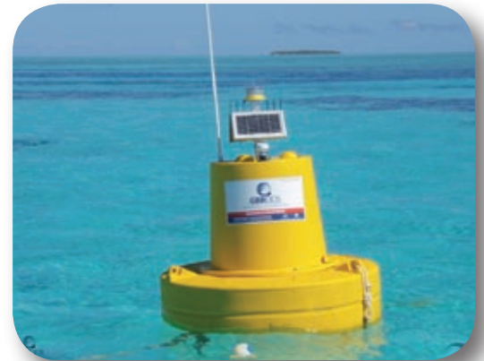
Buoys collect data from the sensor network and sends data back to the main network hub
